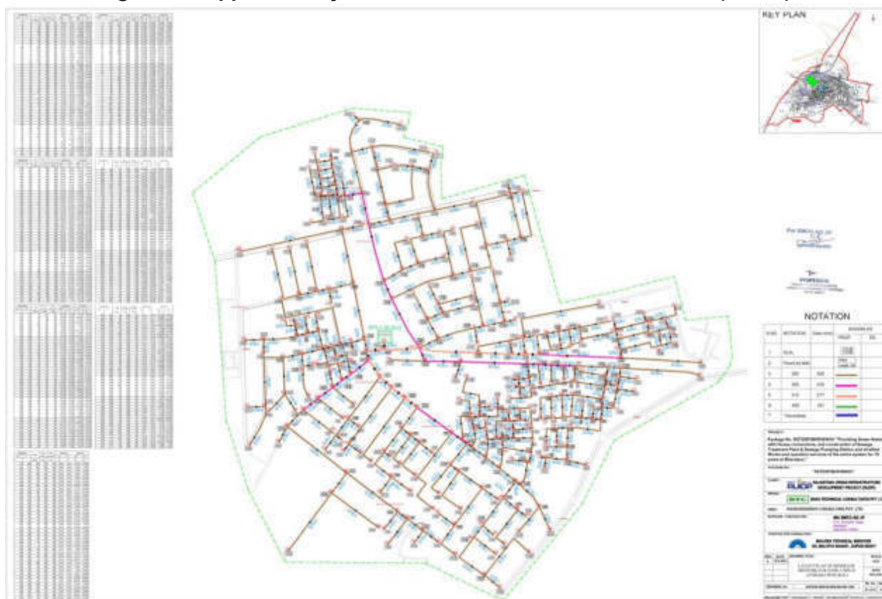
Figure 15: Approved Layout Plan of Sewer Network for Zone-3 (SPS-3).
