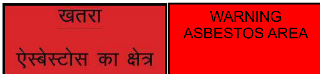
Fig. 3- ACM: In-situ storage warning
