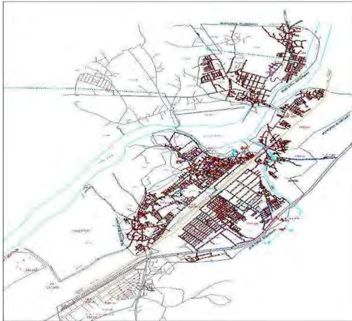
Figure 4: Proposed Water Supply Improvements in Abu Road
