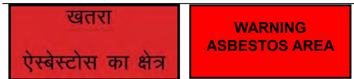
Figure 4: ACM: In-situ storage warning
