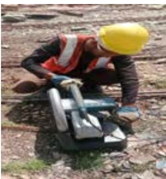
Good Practise: Use Of PPEs & Grinding Machine with safe Guard
