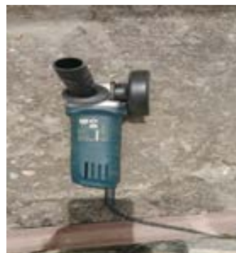
Good Practise: Use Of PPEs & Grinding Machine with safe Guard
