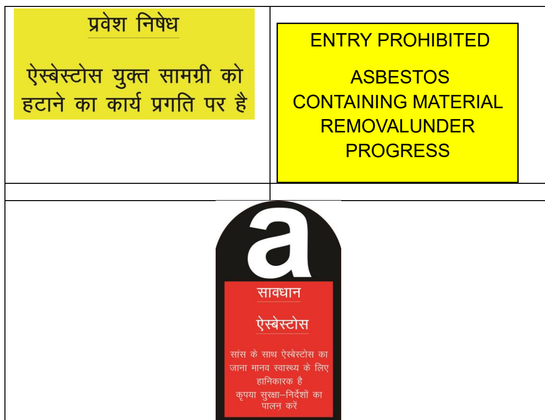
Fig.No.2 Asbestos warning signage
