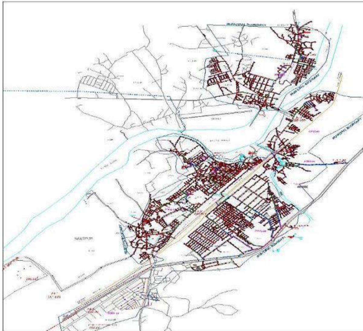
Figure 4: Proposed Water Supply Improvements in Abu Road
