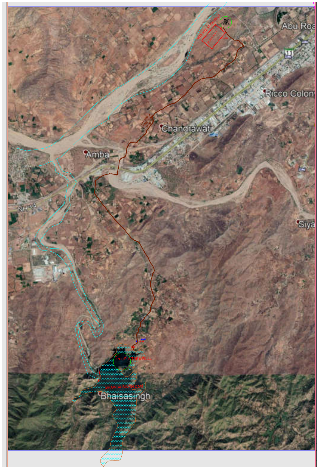
Figure 3: Raw Water Alignment from Dam to WTP
