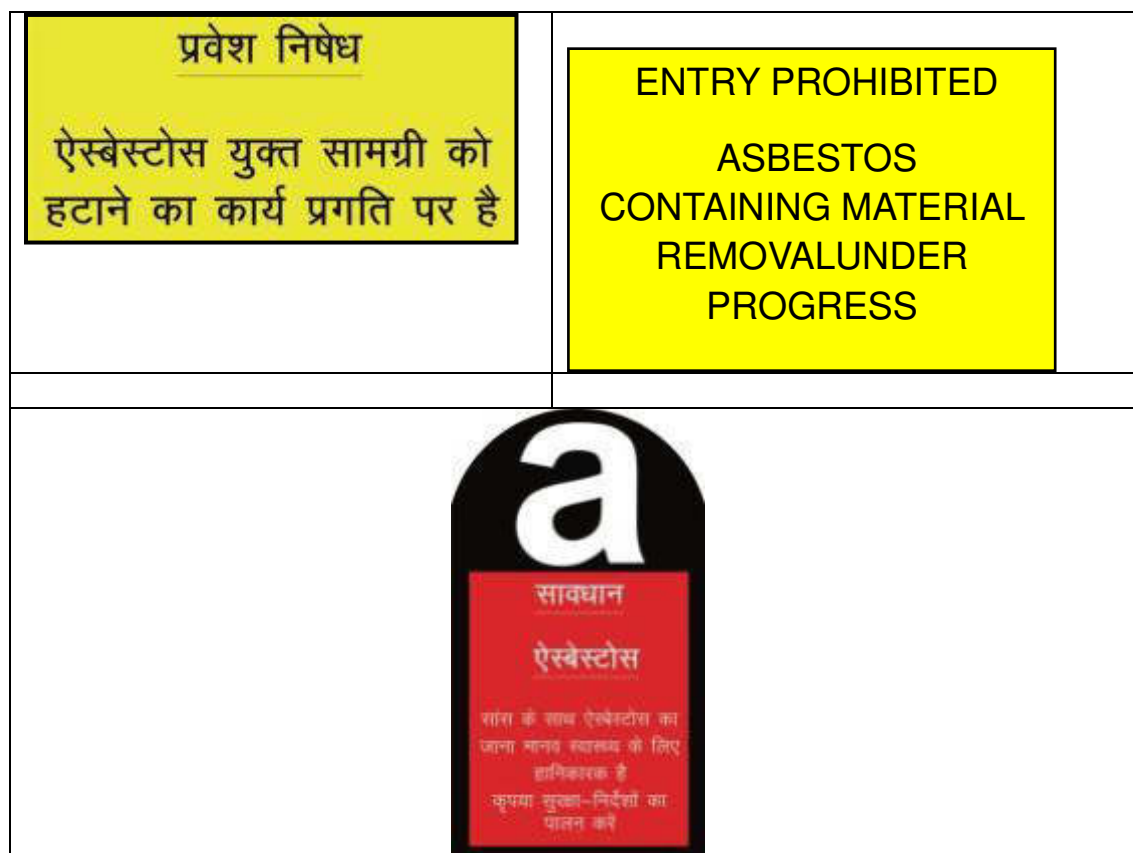
Fig.No.2 Asbestos warning signage
